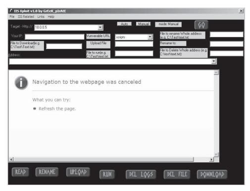
Figure 2-3 IIS Xploit allows hackers to exploit the directory traversal vulnerability in IIS.
